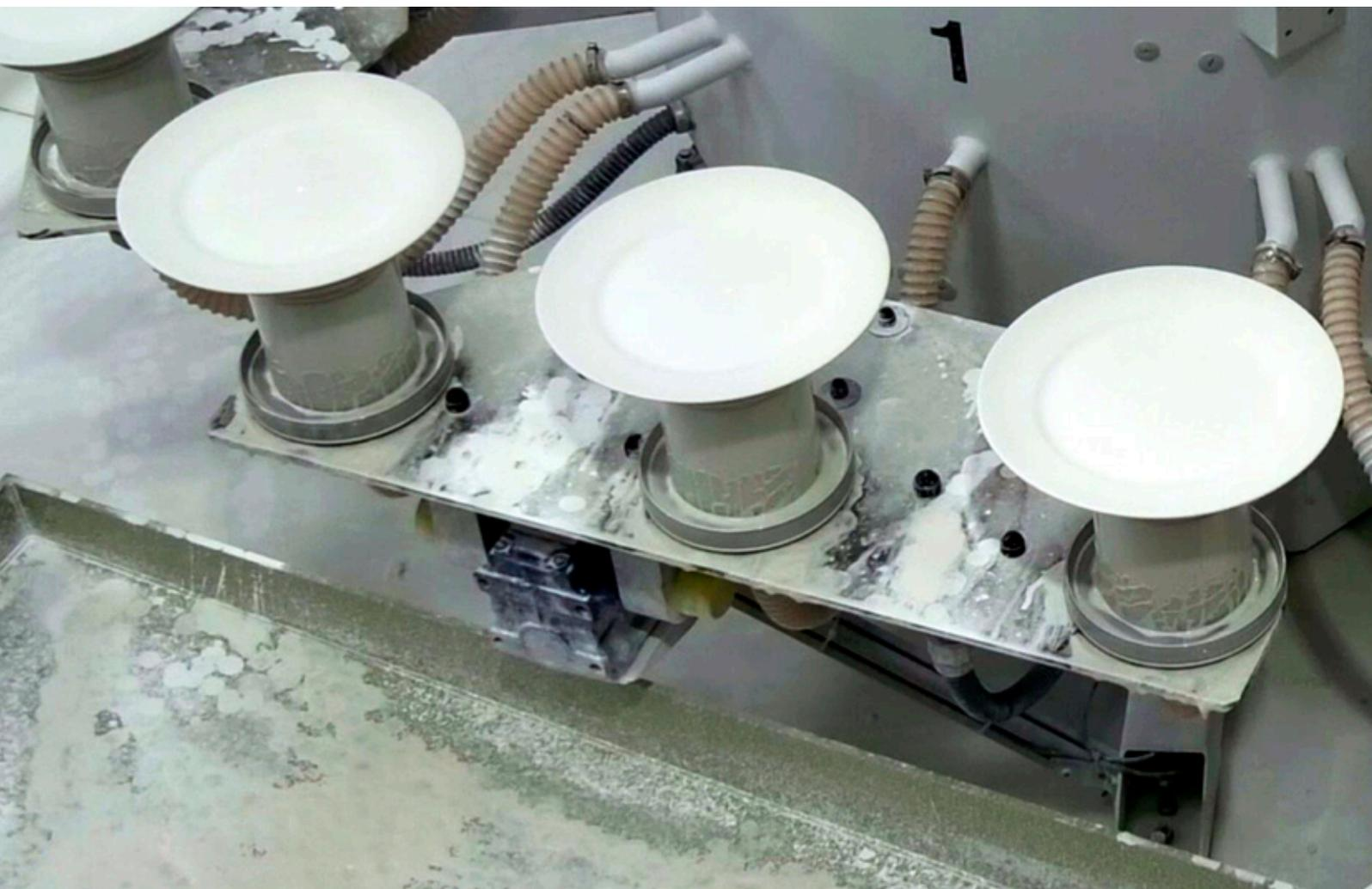
into automated industrial systems - SAMA provides **DUO**, a **highly versatile** stand-alone machine suitable for glazing all types of article and **ideal for testing and small lots**.
