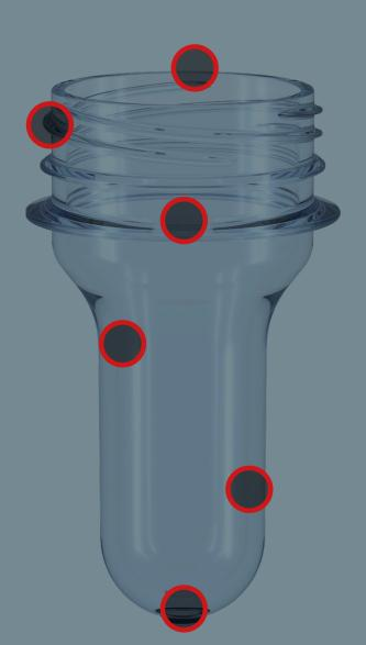
**TOP SEAL:** Contamination, Flashes, Short shots, Notches, Black specks, Indicative measurement of inner and outer diameter, Ovalization
